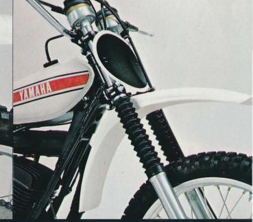
Yamaha's exclusive air cushioned front forks soak up sharp jolts without bottoming. Light weight polypropylene fenders are virtually unbreakable and conical hubs help reduce unsprung weight.
