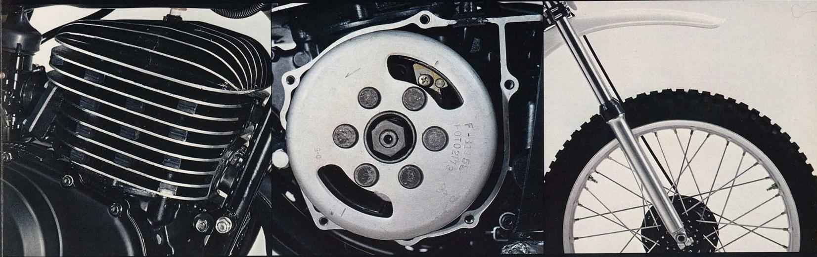
Radial fin cylinder head is designed for better, more efficient cooling.
