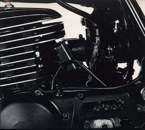
Torque Induction, Yamaha's unique intake system, utilizes a reed valve to feed the engine the exact amount of fuel and air it needs. The result is more horsepower, particularly at low rpm's. The crankcase cover is made of magnesium to reduce weight.
