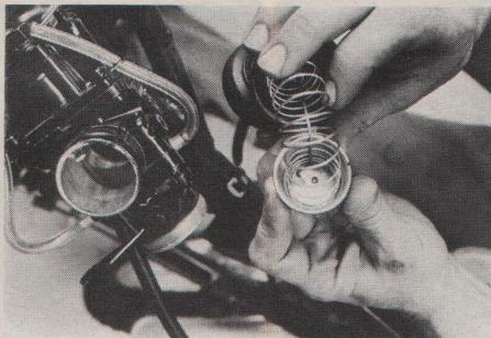
When needle position is changed, be careful not to let clip plate hang up.
