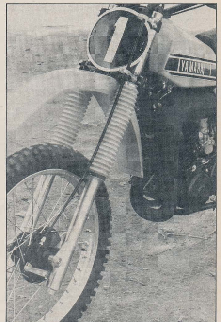
Some of the very finest production forks available. Travel is a full 250mm or 9.84 inches.
