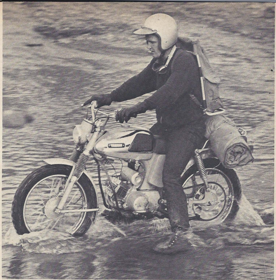
Waterproofing of the ignition system is very good. The Trailmaster will run until the air intake is under water.
