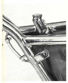
Oil for the Yamaha Autolube Injection System is carried in the frame members. The small plastic tube at the left allows the owner to visually check the capacity of the "oil tank."
