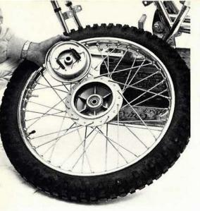
Externally, the braking system on the Rickman Chassis Kit appears to be a bit on the skimpy side. An examination of the internal components, along with a ride on the machine, indicates that the stopping system is more than just adequate. Sealed bearings used in the Rickman wheels do much to reduce down time and maintenance.
