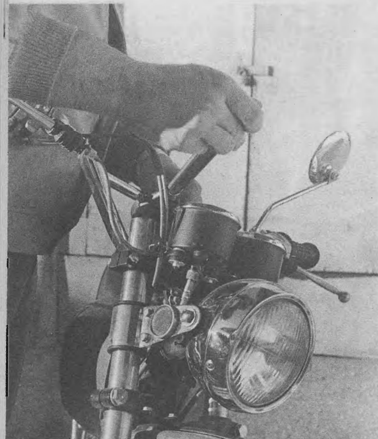
1. Remove the large plugs at the top of the fork legs. This will permit the oil to flow free when the drain plugs are removed.
