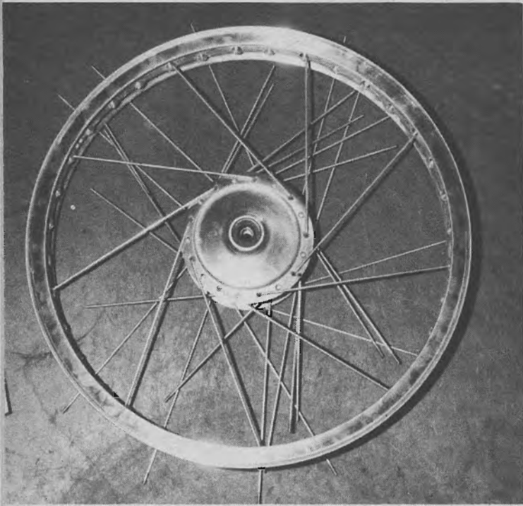
6. When lacing the wheel all the spokes must first be put through the hub. Lay it on a flat surface and begin by putting the top nine (or ten if it's a 40 spoke rim) spokes through the proper hole in the rim. Use another wheel as a guide if necessary.
