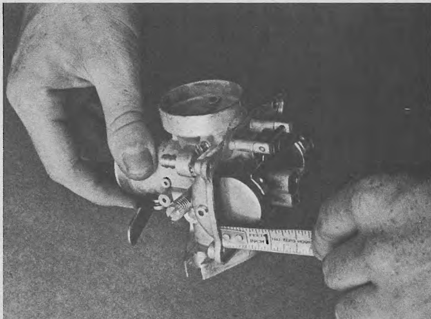
1. Before any tuning is attempted, the float level should be checked and made right if necessary.
