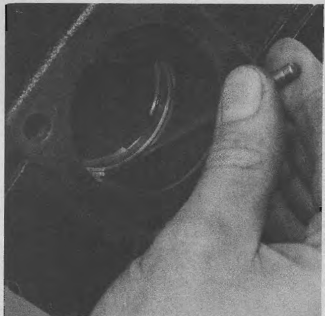
6. Use a machinist's scribing tool or an icepick-like pointer to scribe the lines that indicate the maximum size of the yet-to-be-enlarged ports.
