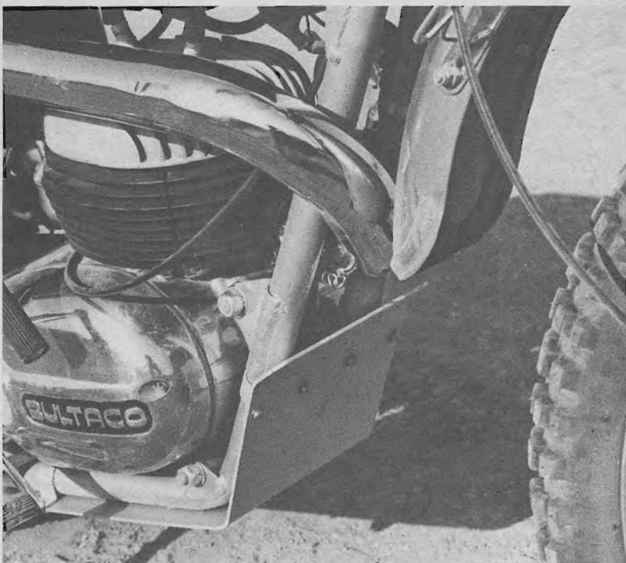
The double loop frame protects the engine but the addition of the skid plate guarantees rocks won't damage the cases.
