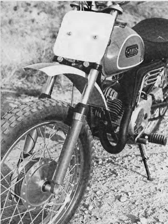
With the addition of heavier weight oil the front forks should work better than the stock arrangement.
