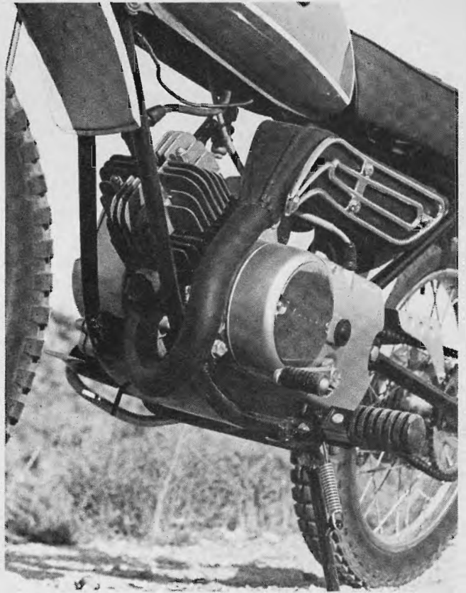
A small engine guard is provided. For most off-road work it should be enlarged to protect the rest of the engine.
