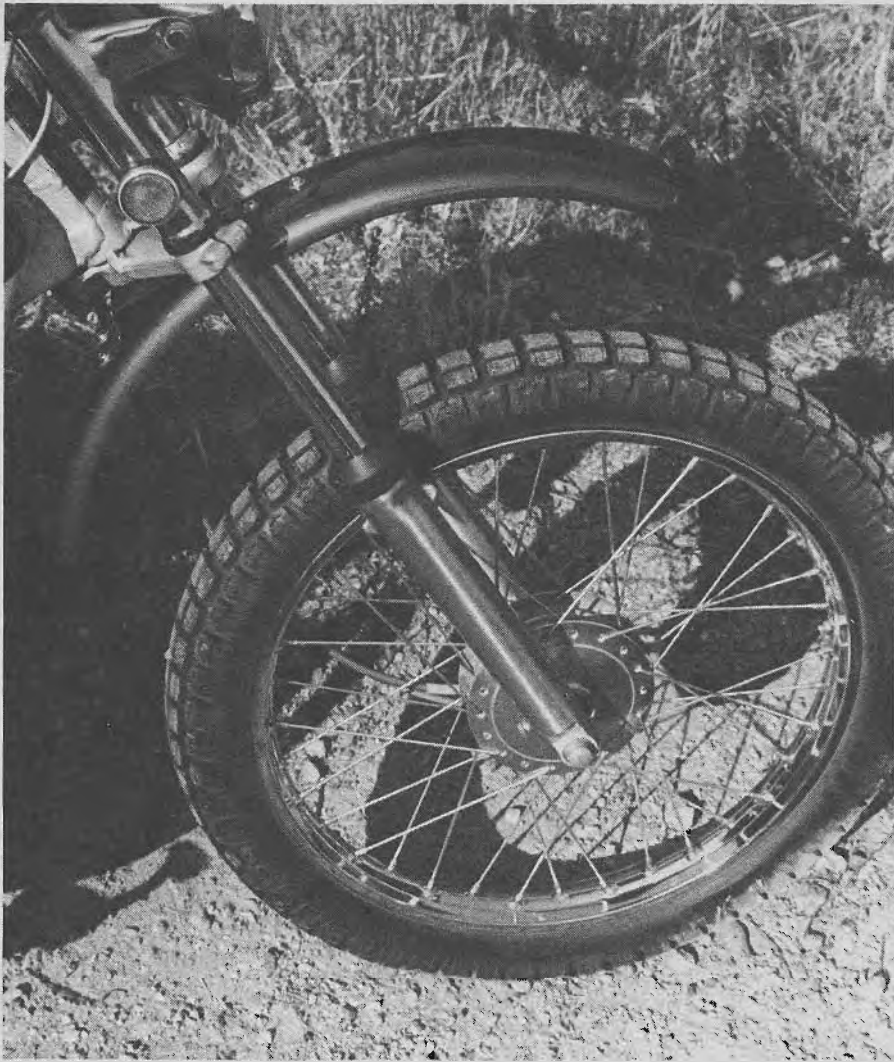
The front forks have over five inches of travel and are dampened very well for a Japanese machine.
