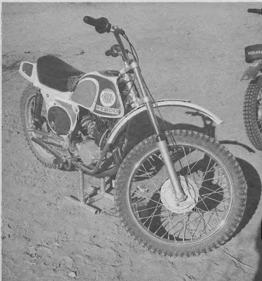
Slim seat and two-gallon gas tank that are standard on "Super Rat" will make the "Ace 100" Hodakas more comfortable for short races and rides. Stock "Ace 90, 100, or 100B" tanks hold 2½-gallons.
