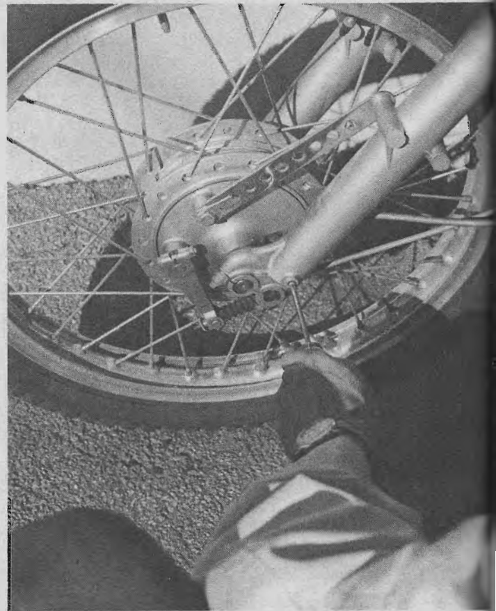
2. Remove the oil drain plug at the bottom of the fork slider.
