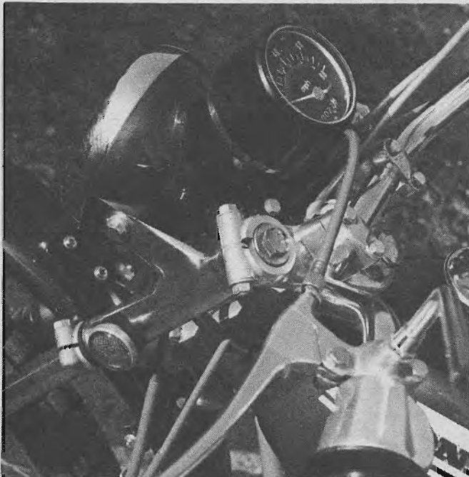
Both the headlight and the speedometer are of the quick-disconnect type so they can be easily removed for serious dirt riding.
