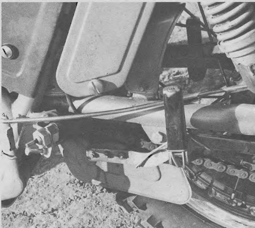
Like Bultaco's trials machine the Montadero incorporates a chain tensioner on the drive chain. Having no slack in the chain provides better throttle response.
