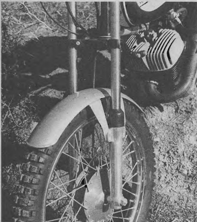
Ceriani forks are used in conjunction with a 21-inch front wheel. The fender should be pulled up to under the fork clamp.
