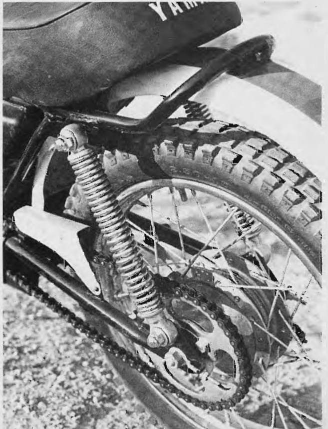
On our test machine the grease-dampened rear shocks were mounted upside down. Perhaps they'll work better when mounted right-side up.
