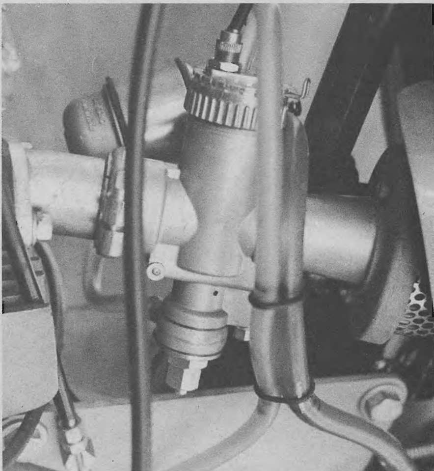
A 24mm Dell 'Orto remote bowl carburetor comes stock. More power can be found by using a larger jug.
