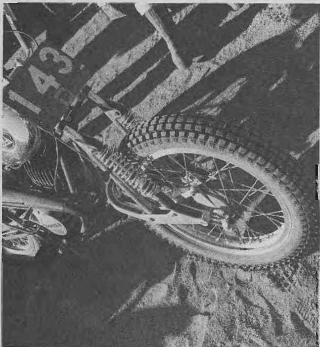
Suzuki Fun Center offers this Van Tech-built leading link front fork to bolt right on to any Hodaka model. "Springer" fork, as they're called, is one of the best for smoothing chuck holes and sharp dips.
