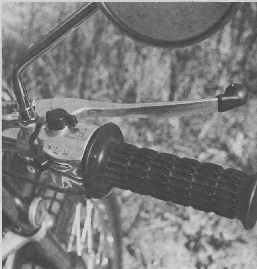
In the Honda tradition a kill switch is located just above the headlight switch.
