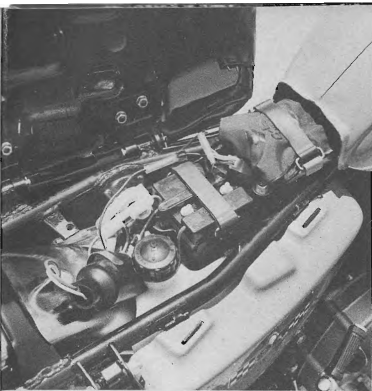
Under the seat will be found the battery, oil tank filler and tool kit. The wires from the taillight can also be unplugged under the seat.
