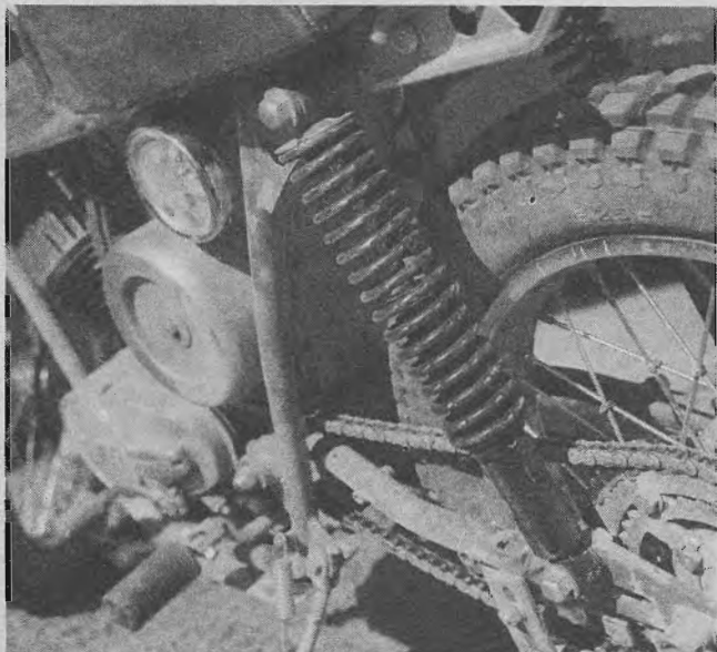
Heavier rear shocks and springs are necessary for fast off-road riding with the Hodaka "Ace 100" models. Every shock maker offers units that'll fit the Hodaka — these are Girlings.
