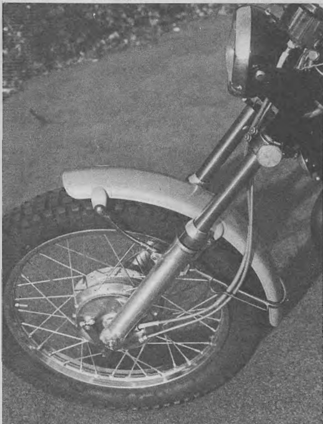
The forks are better than they've been in the past but for serious off road riding the dampening rates must be changed.
