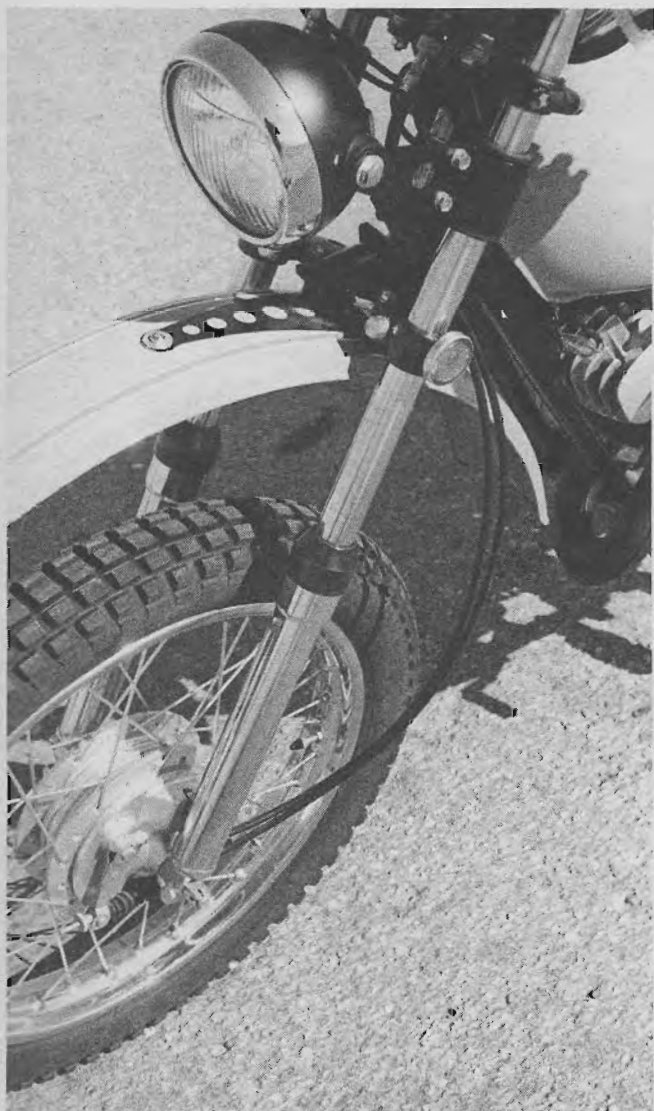
Hatta forks are featured on the Enduro. The headlight is a quick-disconnect, so the rider can take it off if he is so inclined.
