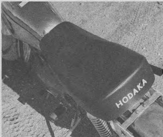
Slim seat and two-gallon gas tank that are standard on "Super Rat" will make the "Ace 100" Hodakas more comfortable for short races and rides. Stock "Ace 90, 100, or 100B" tanks hold 2½-gallons.
