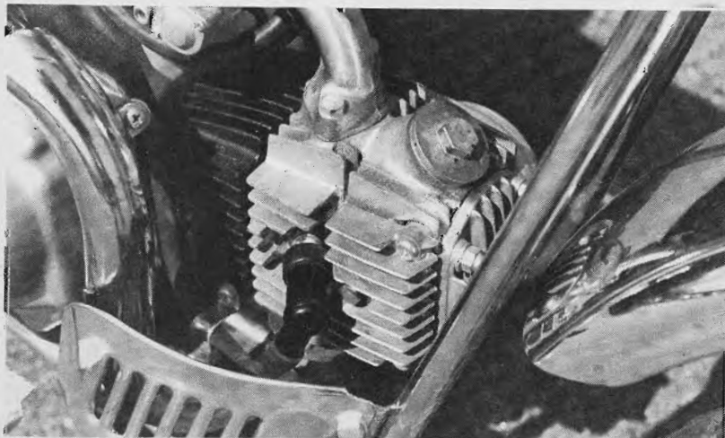
The engine is the typical single cylinder overhead cam unit that Honda uses for all their machines under 100cc.
