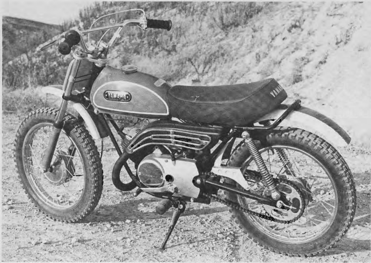
In reality the muffler is concealed in a covering that looks like an expansion chamber.
