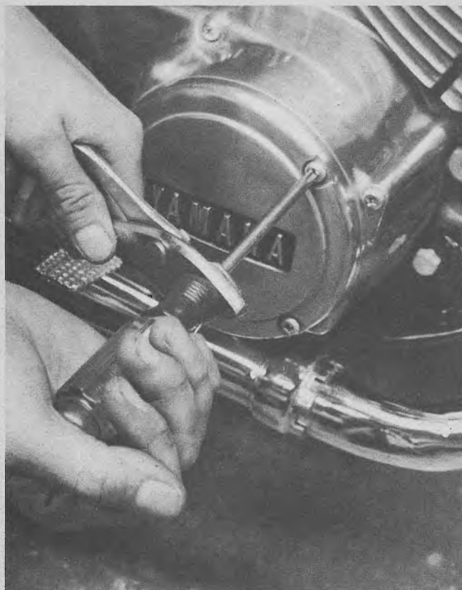
That pair of pliers can be used to give the added leverage needed to break loose most screws, particularly those that hold the ignition point's access cover in place.
