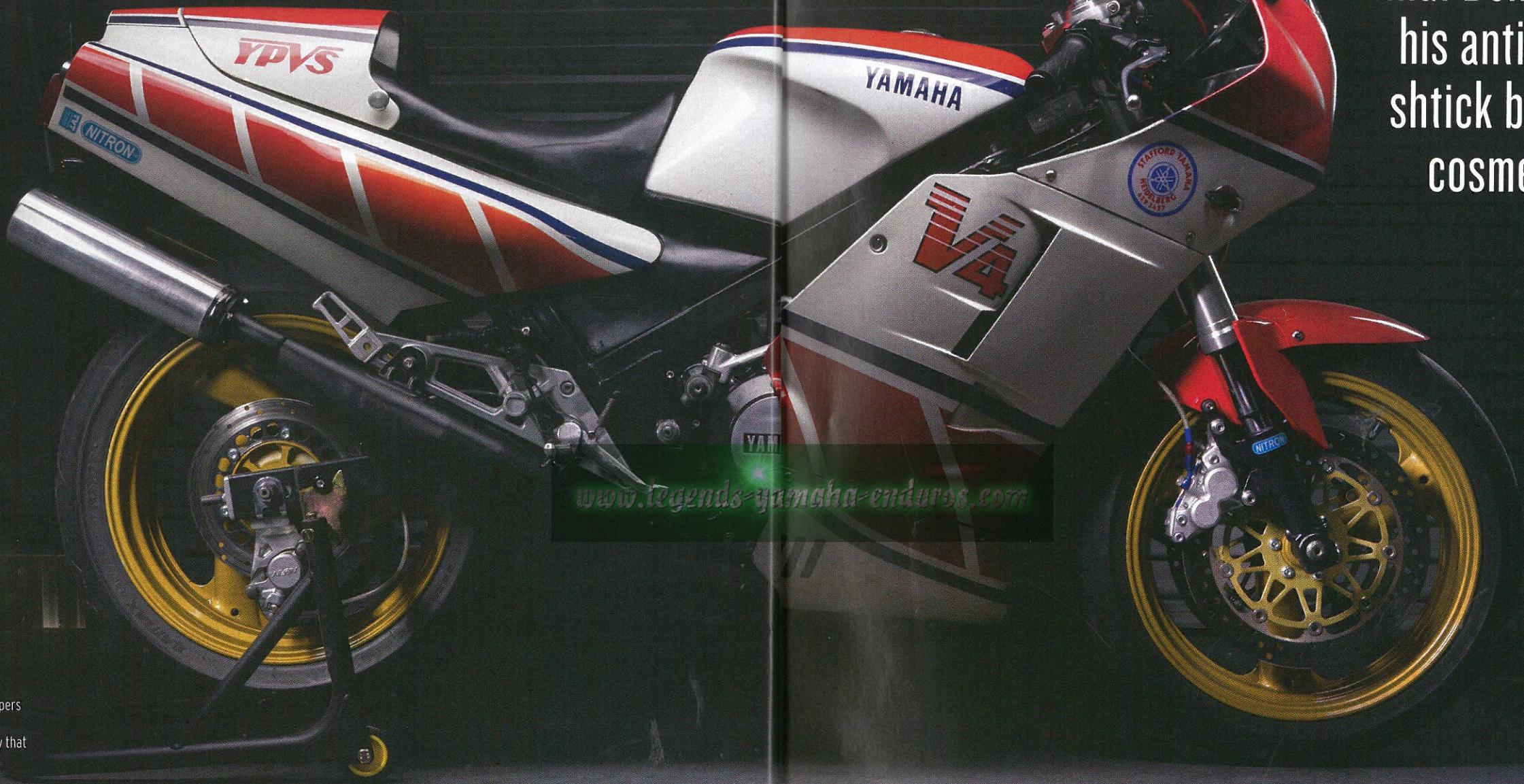
1. The FZR1000 four-spot calipers run smaller leading pistons. Braided hoses are a giveaway that this bike is not standard.
