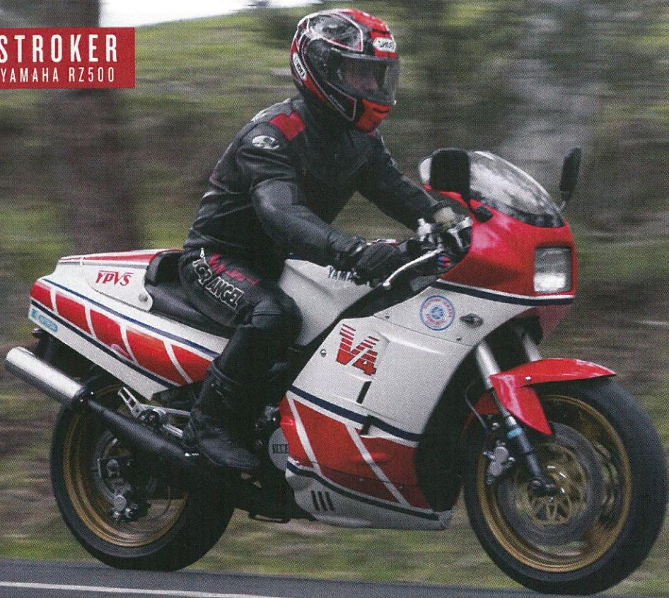
1. R6 clip-ons have been mounted below the top triple-clamp, but the riding position is not that radical.
