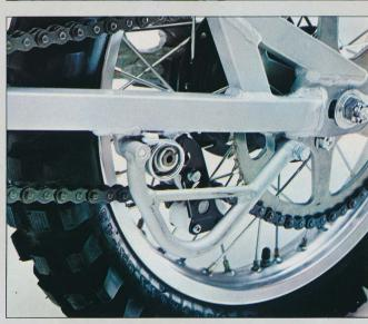
**Long-travel suspension** requires a chain tensioner. The improved design on the new YZ125E keeps the proper tension and reduces chain snap.
