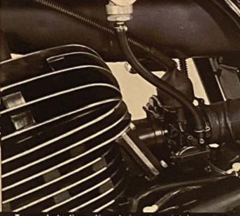
Torque Induction, Yamaha's unique intake system, utilizes a reed valve to feed the engine the exact amount of fuel and air it needs. The result is that horsepower is increased, particularly at low rpm's.
