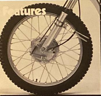
Racing design conical front hub, new spoke and rim design and larger front brake drum combine to make a stronger, lighter, more dependable machine.
