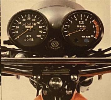
Enduro-type instruments include speedometer, tach, and resettable trip odometer. A single key locks ignition, forks, gas, cap, and accessories compartment. Complete lighting system makes Yamaha Enduros
