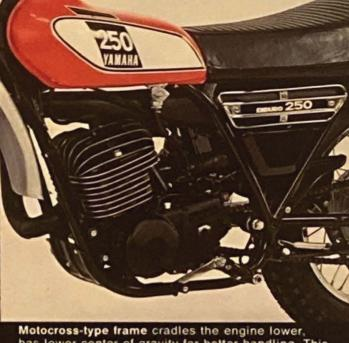
Motocross-type frame cradles the engine lower, has lower center of gravity for better handling. This frame design, adapted from the highly successful Yamaha motocrossers, also flexes less, for surer tracking.
