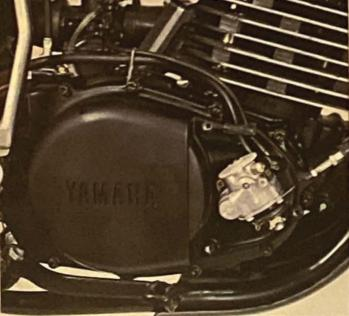
Autolube, a feature on most Yamaha two-stroke engines, automatically injects oil into the fuel mixture, eliminating the need for premixing. And, since it adjusts the flow of oil to engine load and speed, it extends engine life.
