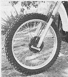
Flimsy front end is weak point of all Yamaha line of dirt racers. Factory bikes use heavily knurled hubs of greater diameter and much stronger clamps.
