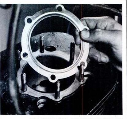
The head gasket goes on next. Place the raised portion down against the cylinder. As with the cylinder, tighten the head nuts evenly and in steps until 18 ft.-lb. has been reached.
