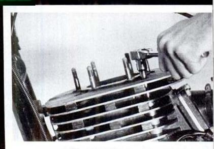
Again using the ratchet, extension and 13mm socket, loosen and remove the four nuts that attach the cylinder to the crankcase. www.legends=yamaha=enduros.com
