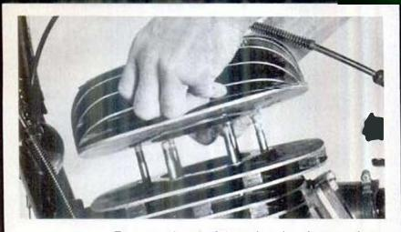
Remove the six 13mm hex-head nuts using a socket and ratchet with a 3-in. extension. It is best to use a magnet to remove the washers on the studs before the head is removed. It is also good practice to loosen the plug before lifting the head off.
