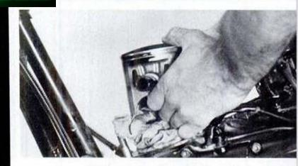
Firmly grasp the circlip with a pair of needlenose pliers. Twist to the inside and at the same time pull out; the clip will come right out. Using a pocket knife or similar tool, deburr the piston-pin hole (above steps not shown), and push the pin out from the opposite side.
