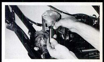
Work the piston pin back and forth through the piston several times to assure a smooth slip fit. Lubricate the small-end bearing and place it in the connecting rod. Install one circlip in the piston with the open end facing the top or bottom of the piston. This way the forces acting on the clip won't have a tendency to close it and pop it out of its groove. Push the pin into the piston and install the other clip in the same manner. Make sure the arrow on the piston crown is facing forward.
