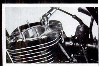
Using a criss-cross pattern, tighten the cylinder nuts to 32 ft.-lb. Start at 15 ft.-lb. and work up from there. This assures that the base will not be tightened unevenly and eventually warp from the heat.
