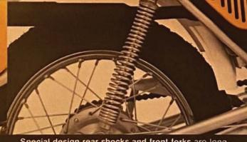
Special design rear shocks and front forks are longtravel units with soft damping characteristics to maintain control on rugged terrain. And to help the wheels ride up over high obstacles easily.
