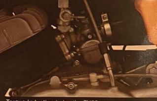
Torque Induction helps the TY80 generate more low speed torque by feeding the engine exactly the amount of fuel and air it needs. Large flywheel design also helps make for excellent low speed control.
