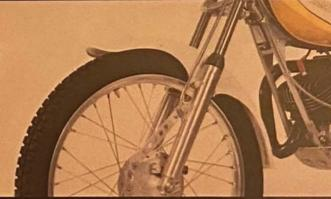
Trials front forks have extremely soft damping action. Hubs and rims are alloy. Fenders are polypropylene. Even the Autolube tank is lithtweight nylon.
