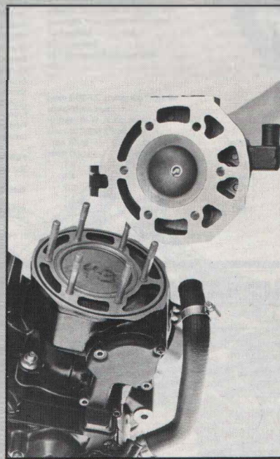
Two O-rings replace a copper gasket
