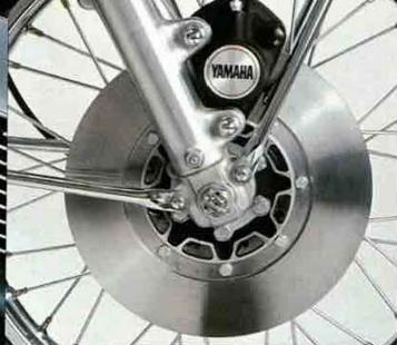
Front disc brake stops you faster. An adjustment screw lets you set the hand-lever for the exact "feel" you prefer. The enduro-type front forks will soak up the hardest jolts and resist bottoming.
