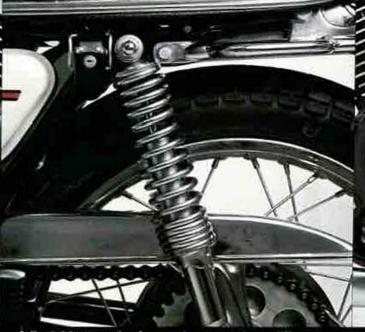
Adjustable rear shocks can be set at three different positions, according to the load you're carrying or the condition of the road. Yamaha's brakes have traditionally set the industry standard for sure stopping.
