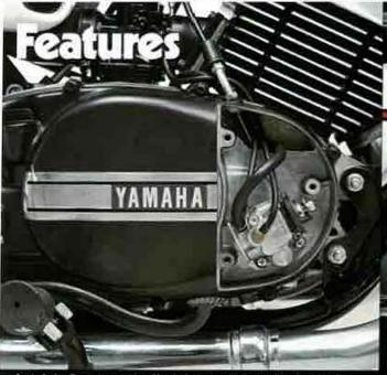
Autolube" automatically injects oil into the fuel mixture, eliminating the need for premixing. And, since it constantly adjusts the flow of oil to engine load and speed, it helps extend engine life.
