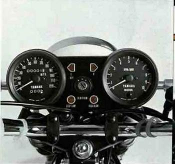
Complete instrumentation includes fully illuminated speedometer, tachemeter, and resettable trip odometer. Ignition key also locks accessories compartment, helmet hanger, steering handle, and gas tank.
