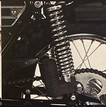
Thermal-Phase rear shocks have built-in oil coolers to prevent overheating, no matter how hard or long you ride.
