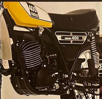
Motocross-type frame cradles the engine lower, has lower center of gravity for better handling. This frame design, adapted from the highly successful Yamaha motocrossers, also flexes less, for surer tracking.
