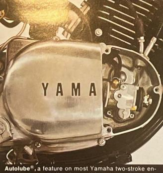
Autolube®, a feature on most Yamaha two-stroke engines, automatically injects oil into the fuel mixture, eliminating the need for premixing. And, since it adjusts the flow of oil to engine load and speed, it extends engine life.
