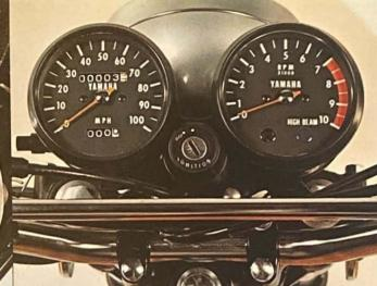
Enduro-type instruments include speedometer, tach, and resettable trip odometer. A single key locks ignition, forks, gas cap, and accessories compartment. Complete lighting system makes Yamaha Enduros fully street legal.
