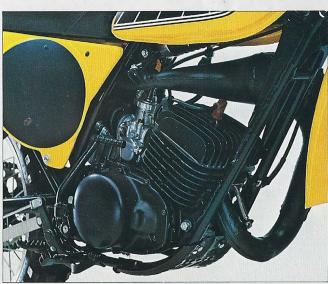
Center-mount exhaust system is routed out of the way, under the padded saddle, for more protection from road obstacles. A tuned silencer reduces noise without affecting performance.
