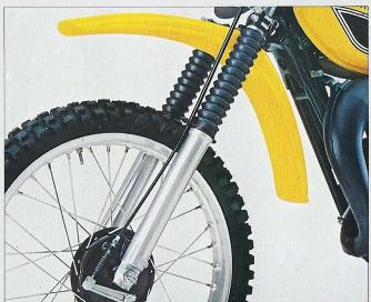
Heavy-duty front forks are air-cushioned, with long travel for soaking up bumps. Alloy rims and conical front hubs reduce weight and the lightweight polypropylene fenders are virtually unbreakable.
