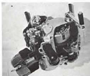
Autolube is Yamaha's revolutionary oil injection system.
