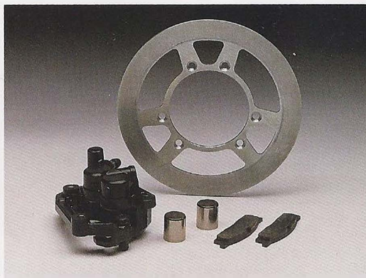
The YZ80 stops as well as it goes, courtesy of a 190mm front disc brake.
