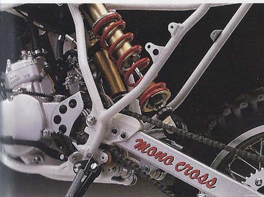
Our smallest YZ's rear suspension is just like our bigger YZ's: a Monocross setup.
