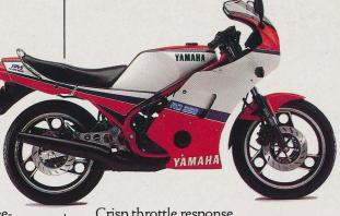
Crisp throttle response throughout the rev range is assured, by the unique YPVS system, which matches exhaust port timing to engine speed, giving one of the widest spreads of power, of any two-stroke, and the smoothest possible mid-range running. So successful is this engine, that it's powering machines, in only a slightly re-tuned state, to victory in Formula II races!
