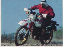
Also common to both models is the superb monocross rear suspension system, with heavy duty, air-assisted, motocross type forks smoothing out the bumps at the front.
