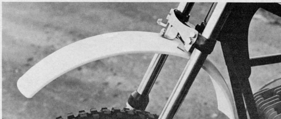
There are a number of plastic and fiberglass front fenders for sale. The Preston Petty front fender pictured here is one of the unbreakable types on the market.
