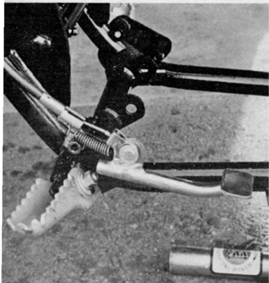
The Rickman Hodaka brake assembly and cable mounts easily to the Champion foot peg bracket. The Champion foot pegs are a copy of the latest Bultaco design.
