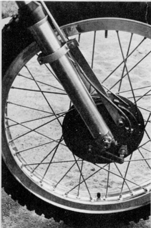
The completed front end is light and strong. The custom torque arm must be fabricated after the slider legs are turned down. The Rickman magnesium brake really works.
