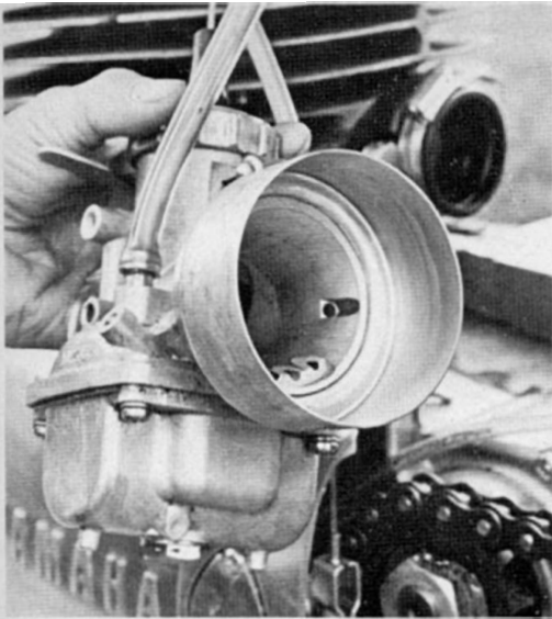
The adaptor fitting by K&N Engineering is essential to allow the 34mm Mikuni road racing carburetor to breathe adequately throughout the entire RPM range.
