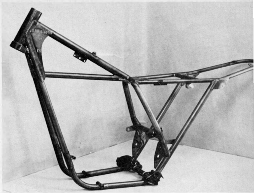
The Champion motocross frame is constructed entirely of chrome moly tubing. Extremely strong, with a proven geometry for excellent handling, it weighs only 17 pounds.
