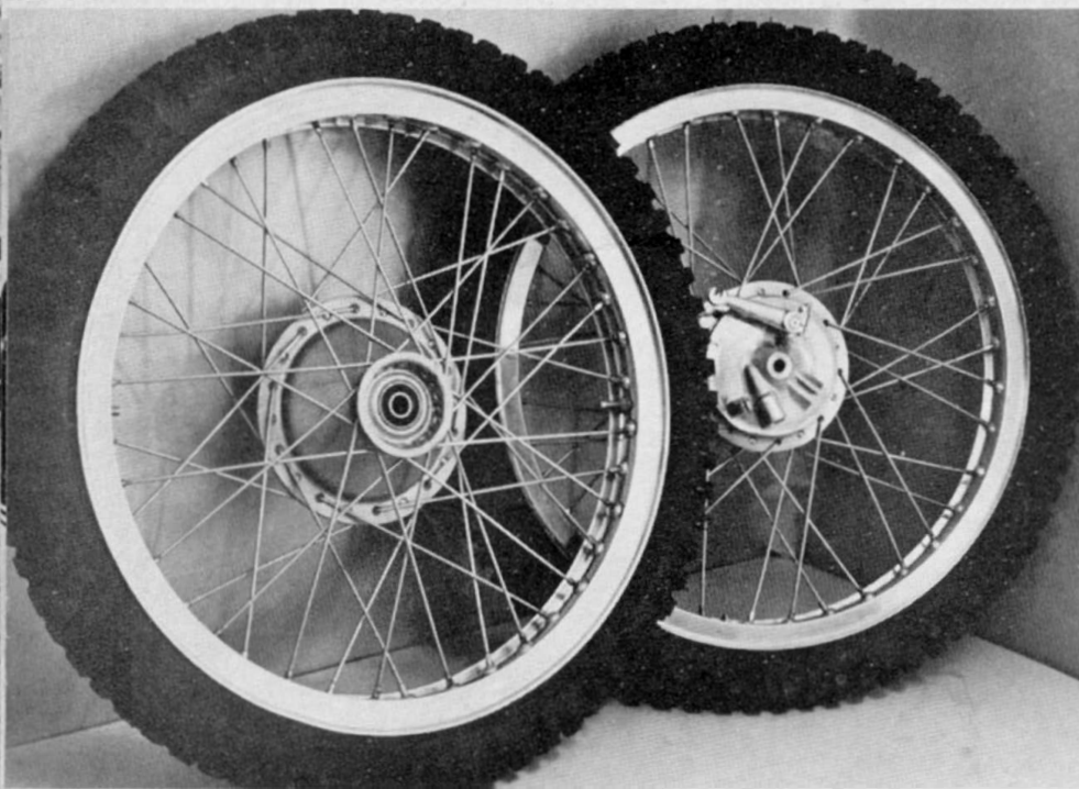
The Yamaha AT1 hub (right) was the lightest motocross unit available. The Rickman magnesium unit (left) is two pounds heavier, but stronger. Baroni MX rims and Dunlop tires are secured with stainless steel spokes.
