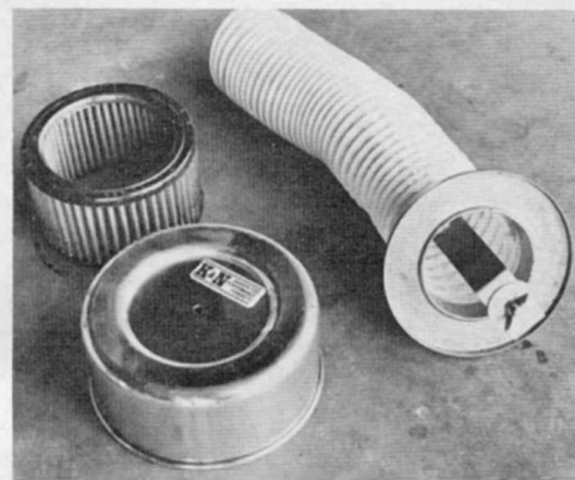
K&N Engineering manufactures this special air cleaner assembly which does not restrict the air flow into the big 34mm Mikuni road racing carburetor.
