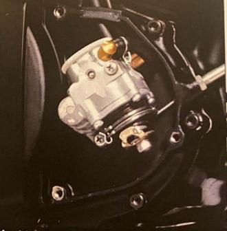
Autolube a feature on all Yamaha two stroke engines automatically injects oil into the fuel mixture, eliminating the need for premixing. And, since it adjusts the flow of oil to engine load and speed, it helps extend engine life.
