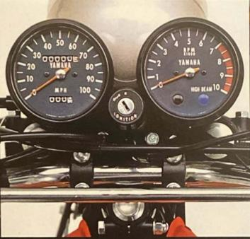
Enduro style instrumentation includes speedometer, tachometer and re-settable trip meter. Large sealed-beam headlight provides bright, automotive type illumination. Complete lighting system makes Yamaha Enduros fully street legal.
