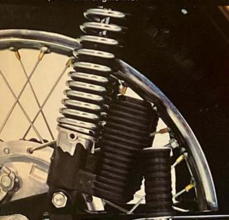
Forward-mounted thermal phase shocks provide greater rear wheel travel for better control, more comfort and consistent traction over rough terrain. Built-in oil coolers help prevent fade caused by overheating
