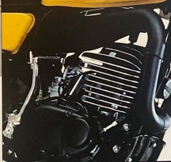
Center mount exhaust system is routed out of the way under the padded saddle. The much narrower profile is more comfortable and allows better control. The tuned silencing system reduces noise without affecting performance.
