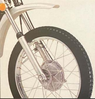
Long travel front forks and 21" front wheel take obstacles and road hazards in stride. Front end steering geometry contributes to precise tracking and positive feel.
