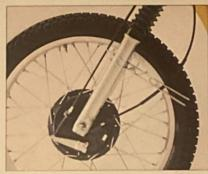
Racing design conical front and rear hubs, spokes and rim design combine with the drum brakes to make the DT 400 a strong, tast and sure-stopping machine.
