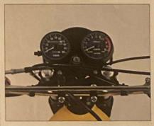
Enduro instrumentation includes a large, sealed-beam headlight, speedometer, tachometer, and re-settable trip meter.
