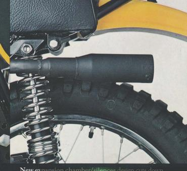
Thermal-Phase rear shocks have built-in oil coolers to prevent overheating, no matter how hard or long you ride. Interchangeable jets also allow you to adjust compression and rebound characteristics individually.
