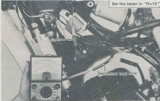
Secondary winding resistance check
