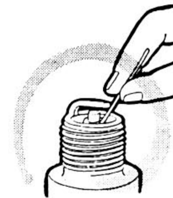
When you do not have a cleaner, clean it with wire or needle.
