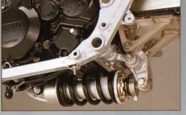
Square section steel frame employs a widely spaced double cradle design with hefty bracing at the steering head and swing arm pivot. The lower right frame section removes to allow easy engine access.
