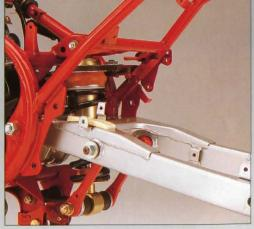
The rising-rate monocross suspension provides the right progressive action for varied surfaces and riding usage. 5 way adjustment is possible by simply turning the remote control adjuster. The lightweight monocross suspension system works together with the new square section swing arm to give the most positive rear wheel tracking ever.
