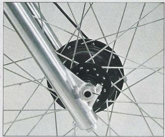
The leading axle design allows quicker, more precise low-speed steering. In addition, the damping characteristics can be improved through the increased oil capacity of the fork tube.
