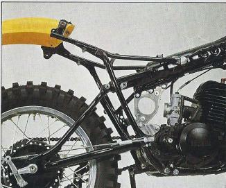
Monocross Suspension allows 9.84 inches of rear wheel travel. New De Carbon type shock absorber allows you to easily and quickly adjust spring preload and damping rate.
