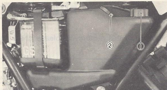
1. Oil tank filler cap 2. Dip stick
