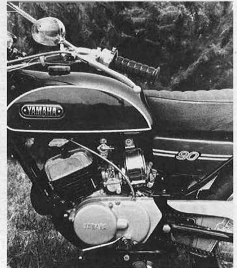
The piston-port engine is a good 90cc slogger.
