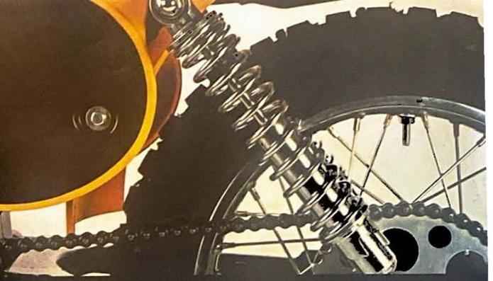
**Forward-mounted shocks** provide greater rear wheel travel for better control, more comfort, and consistent traction over rough terrain.
