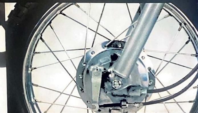
**Large diameter front brake** is water, dust and fade-resistant. Long-travel front forks soak up hard jolts and resist bottoming.
