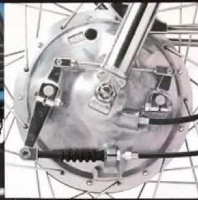
Double leading shoe front brake has tremendous stopping power, and is dustproof and waterproof. The enduro-type front forks will soak up the hardest jolts. Without bottoming.
