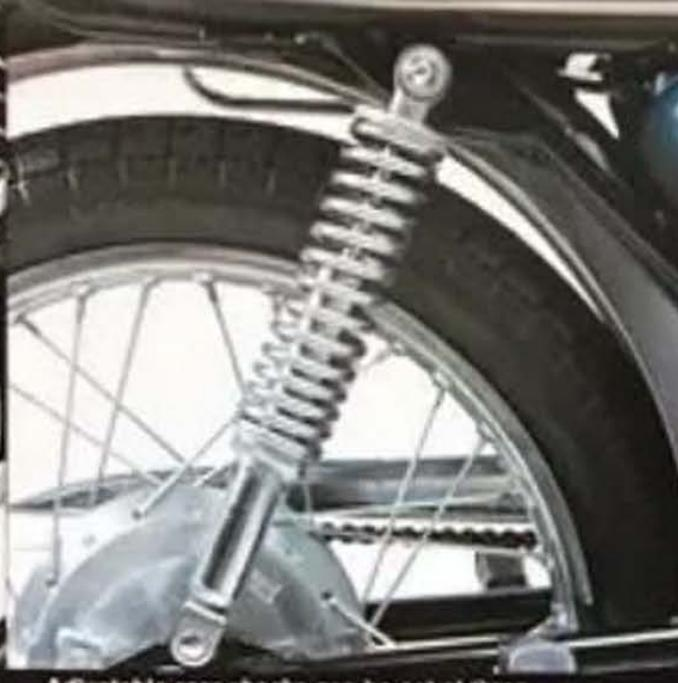
Adjustable rear shocks can be set at three different positions, according to the load you're carrying or the condition of the road. Yamaha's brakes have traditionally set the industry standard for sure stopping.
