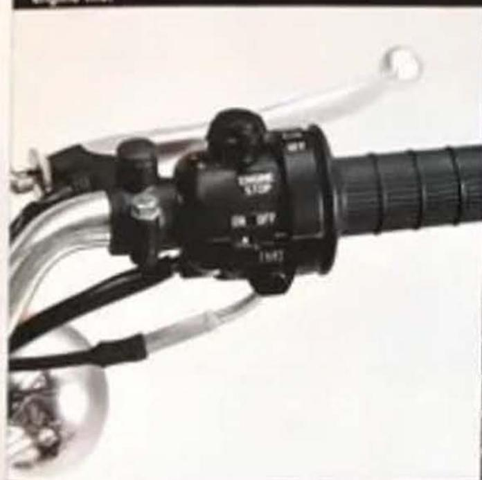
Pushbutton electric starter fires up the RD200's engine at the touch of a finger. Auxiliary kick starter is primary type, so you can start the engine in any gear, without hunting around for neutral.
