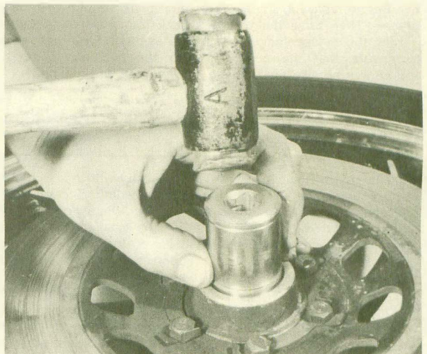
11.5b ... and drive into hub as shown
