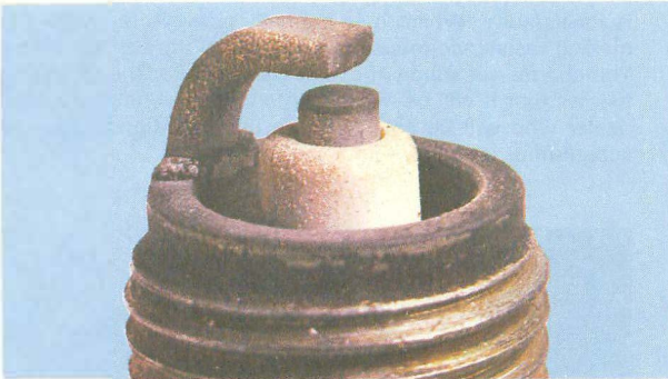
Spark plug conditions: A brown, tan or grey firing end is indicative of correct engine running conditions and the selection of the appropriate heat rating plug
