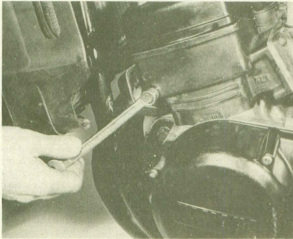
4.4a Remove drain plug and allow coolant to drain
