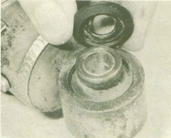
11.5 Mounting bush is protected by end seals
