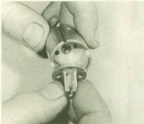
7.8b Lift anchor plate away and displace needle
