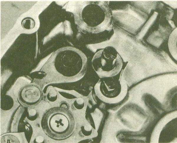
26.5c Assemble stopper arm and tighten pivot bolt
