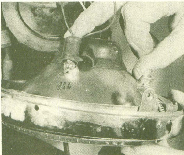
9.4 Pilot bulb has bayonet fitting
