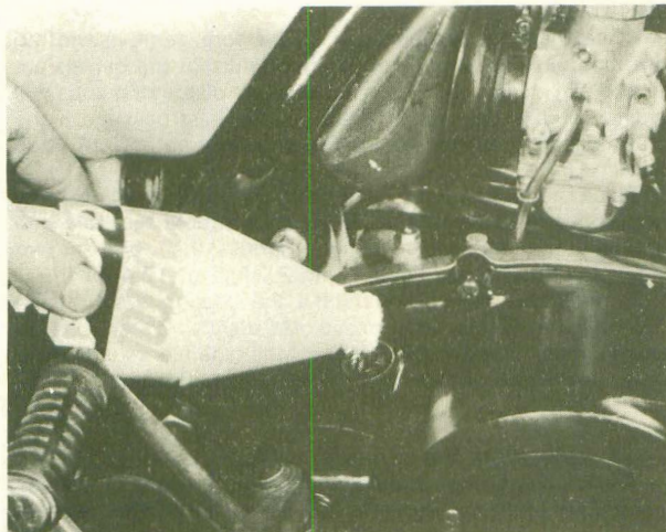
Top up crankcase with SAE 10W/40 oil
