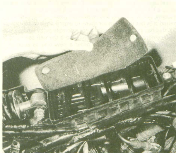
Air cleaner element can be removed for cleaning
