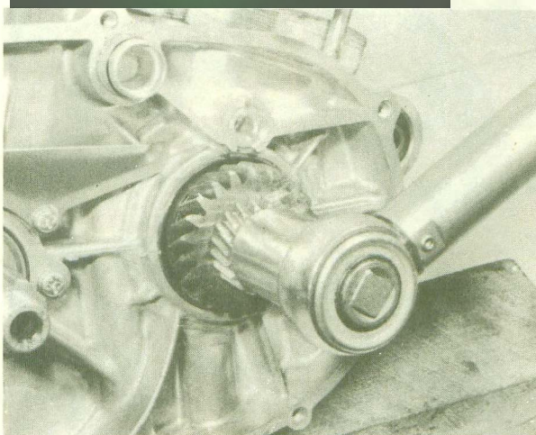
32.2c Lock crankshaft and tighten securing nut
