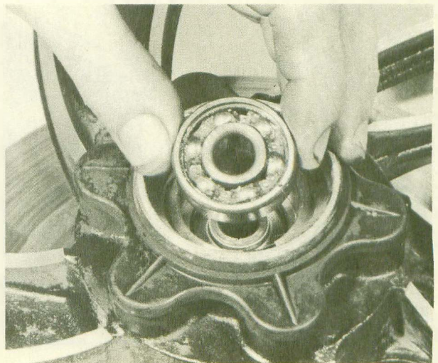
11.5d ... grease and install remaining bearing
