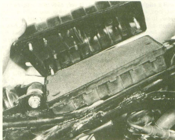
Remove air cleaner cover to expose element
