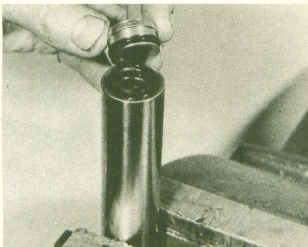
4.1b Remove top plug, if still in position ...
