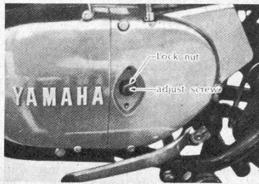
Clutch adjusting screw and locknut (Courtesy Yamaha Int. Corp.)
