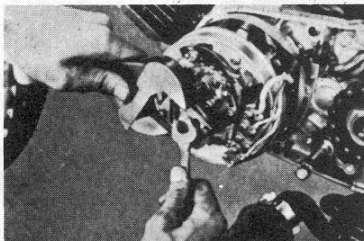
Secure the timing advance weights to remove the armature bolt (Courtesy Yamaha Int. Corp.)
