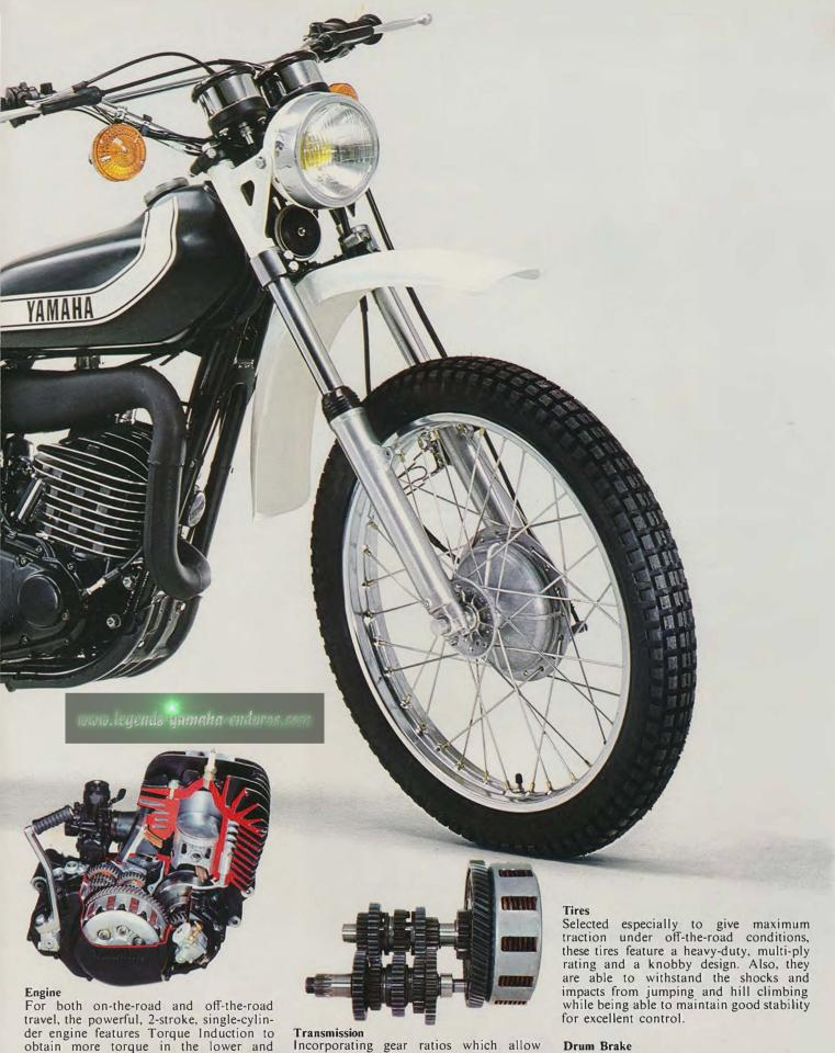
der engine features Torque Induction to obtain more torque in the lower and medium speed ranges thereby yielding a smooth, even response over the entire operating range of the bike. Also, the engine has an aluminum cylinder with cast-iron sleeve for durability and, coupled with the efficient head-fin design, outstanding heat-dissipating characteristics for better engine operation over rugged trails.
