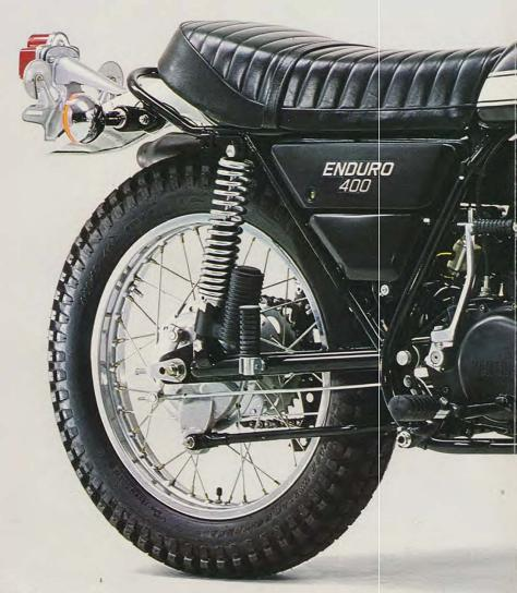
The muffler is routed up from the center of the engine and tucked under the seat in order to maintain the overall slender profile of the bike. This muffler is able to efficiently reduce engine noise without appreciably affecting the high performance characteristics of the engine.
