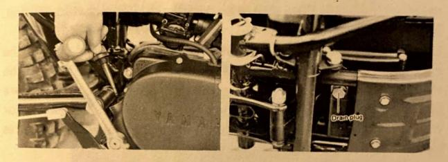
After draining the oil, fully tighten the oil drain bolt, and fill with new oil to the specified level.
