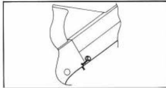
Tank rail drain bolt
