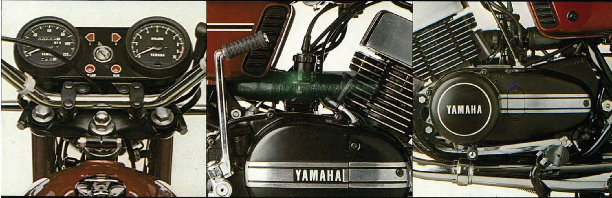
Complete instrumentation includes fully illuminated speedometer, tachometer, and resettable trip odometer. Ignition key also locks accessories compartment, helmet hanger, front forks, and gas tank.
