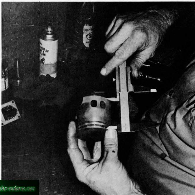
Measure the height of the piston at the edge, subtract 1mm in the calipers, and scribe a line at the skirt.
