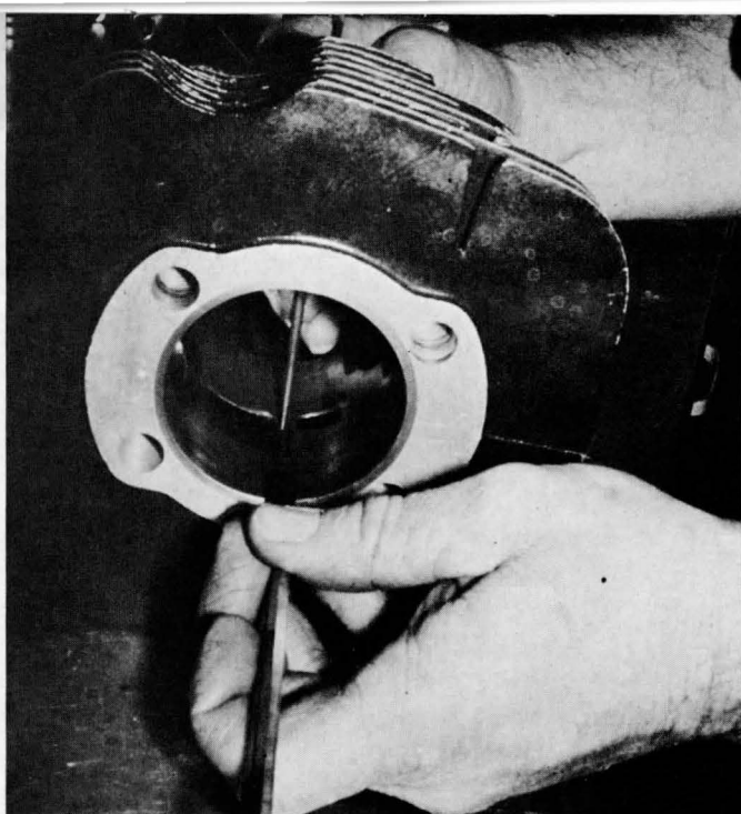
Thin scribe lines are scratched into the Dykem to serve as guidelines for the grinding chore.
