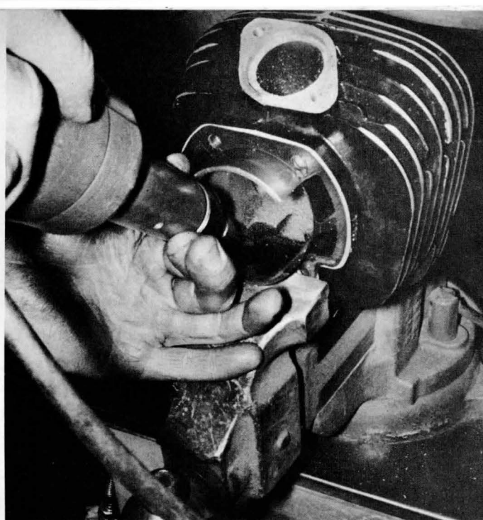
Modifying 2-cycle cylinder ports not only takes special tools but a special talent, also.
