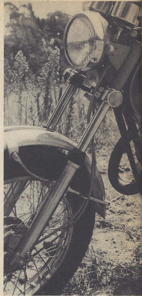
Front suspension is snug yet not hard. No oil leakage is evident.
