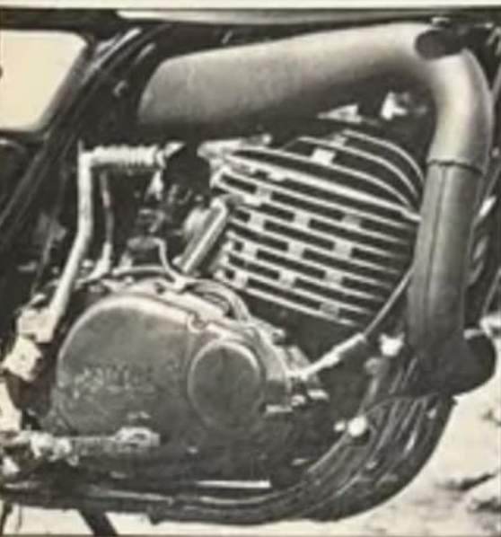
ABOVE LEFT — Over-the-top exhaust system is tucked inside frame. Engine features auto-mix lubrication and reed valve ports. ABOVE RIGHT — Battery, tool kit and engine oil tank (not visible) are accessible simply by lifting seat. TOP RIGHT — Telescoping front fork has internal springs, two-way hydraulic damping and over six inches of travel. RIGHT — Rear brake shoes float unaffected by action of swing arm; note flared reservoir on shock body.
