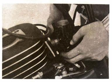
g. Remove the four cylinder mounting bolts so cylinder can removed.
