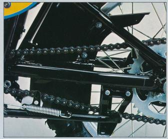
Chain shield keeps mud and sand from being thrown into the chain. Increases chain life.
