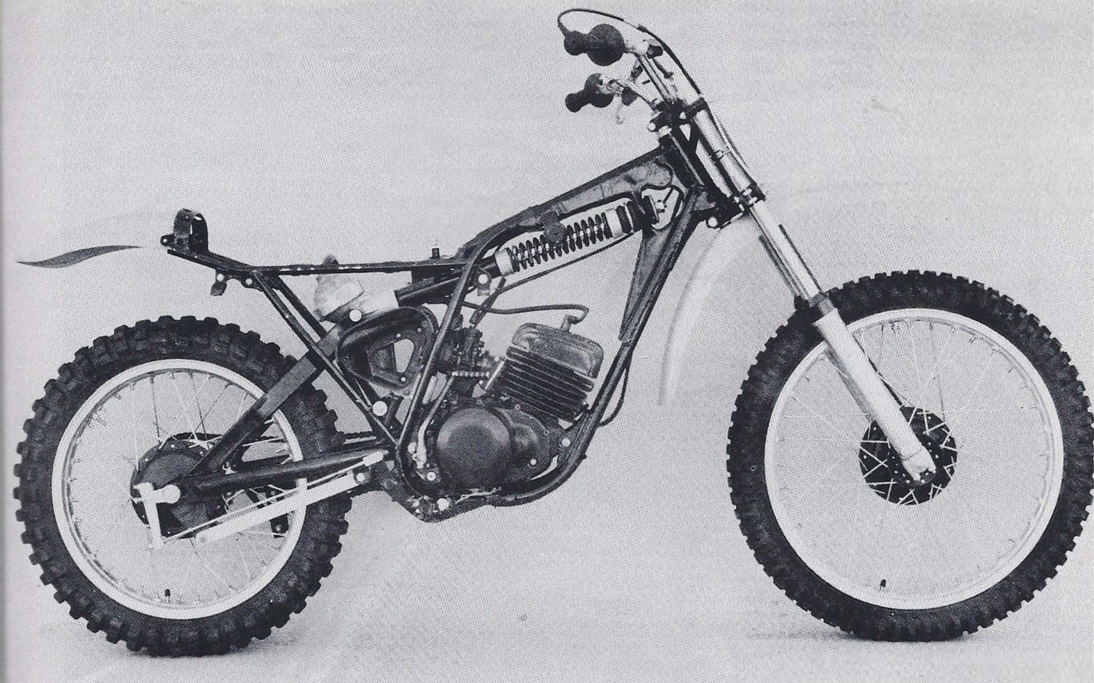
The long, large monoshock unit attaches at the frame head support. The cylinder slides over the piston. Split air filters clear shock unit.
