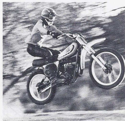
The YZ-C is a rocket with its feathery 193 pound weight (wet) and 20-plus hp engine. Monoshock system is stiff for a light bike.
