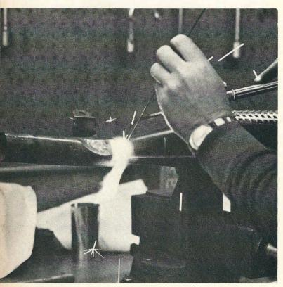
— and then finish off the machine where you can get good access all around the weld area.
