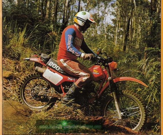
with a weak midrange and bottom end. We fiddled with the PE and came to the conclusion that stock jetting was too rich: down 10 on the mainjet and lower the needle. Much better, but still weak in the lower rev range, enough to make you really con-centrate on hills. It's not that it's too rich on the pilot jet, it's more ignition and pipe.
