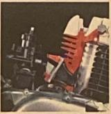
2 Exclusive Yemaha TORQUE INDUCTION means better breething and more horsepower at all rpm's. Reliable stainless steel reed valve between the carb and cylinder opens on engine demand, closes to prevent blow-back 7-port breathing means more power, cooler running.
