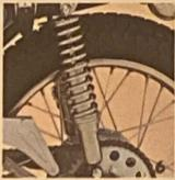
8. For maximum control and riding ease, the rear suspension is equipped with an edjustable 5-position system that ellows the rider to change the tansion of the rear shocks.
