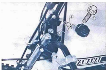
1. Flange bolt 2. Handle upper holder
