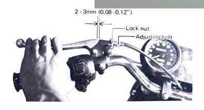
The RD350 has two clutch adjustments. The first adjustment, located at the handlebar lever, is used to take up slack from cable stretch and to provide sufficient free play so that the clutch engages and disengages completely. The picture left illustrates all the parts involved in making the adjustment.
