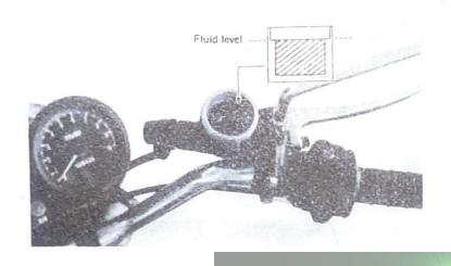
3. Checking the front brake fluid
