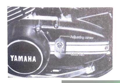
b The second adjustment is located behind the adjusting cover. Removing the cover will expose the adjusting set screw and lock nut.
