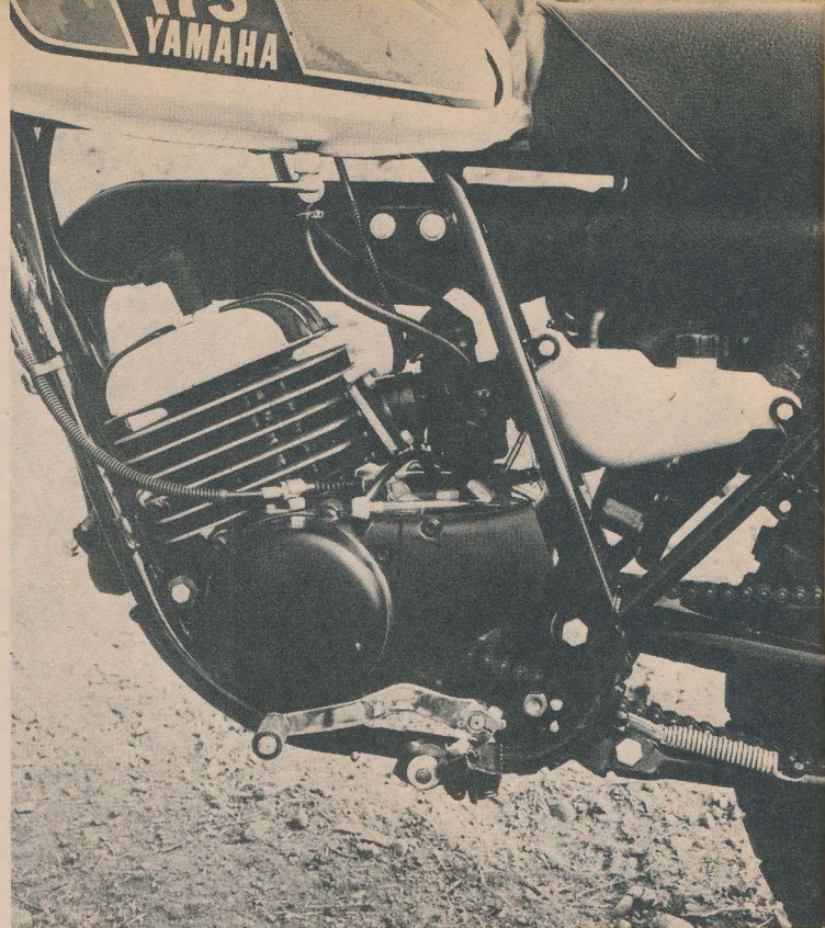
Oil tank is white object above lever, inside side cover. Pipe exits to the right, sweeps to rear left of machine.
